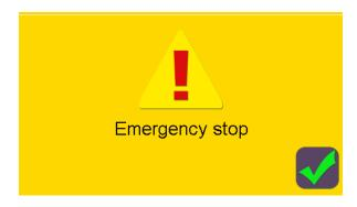
To return to the main menu, turn the emergency stop button and place it in its initial position, then press the icon at the bottom right of the alarm message.
