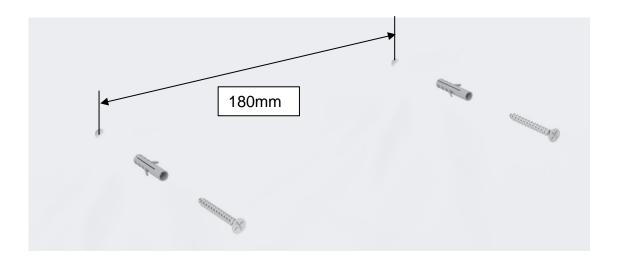
Using a hammer, insert the two plugs and then tighten the screws, leaving them a few millimetres overhanging.
