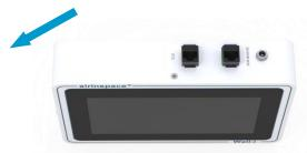
Check the electrical connection of the **Wall-i Watch** to the jack plug (24Vcc).
